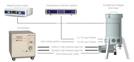
Schematic diagram of Sample Puck Tester system
